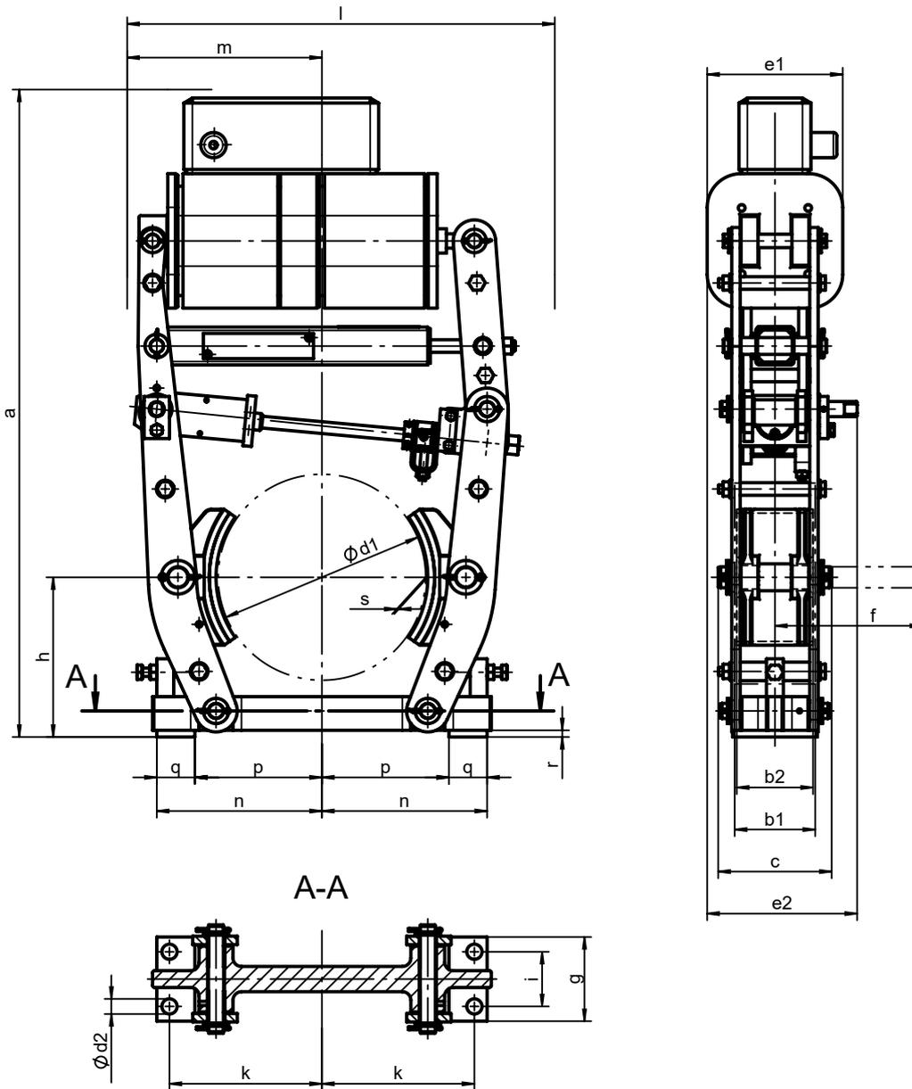
f = required space for removing brake shoe pin
