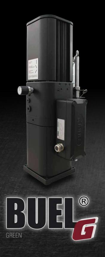
The BUEL® Model G is a new family member of the PINTSCH BUBENZER brand BUEL®. It is a compact thruster to feed active or passive hydraulic brakes and emergency brakes. It is also suitable for small capacity hydraulic cylinders. Operational pressure can be up to 250 bar.
