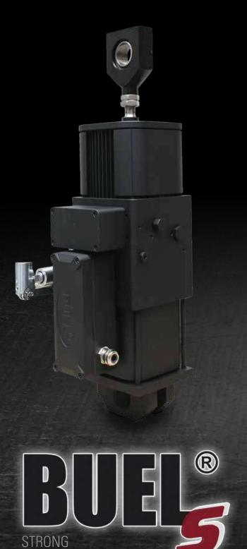
The BUEL® Model S is a brand new family member of the PINTSCH BUBENZER brand BUEL®. It is designed for wheel brakes on rail mounted cranes, where high pulling forces for mechanical wheel brakes are required. The patented cylinder system generates pulling forces up to 40.000 N. It has a robust, but also compact design for rough environmental conditions.
