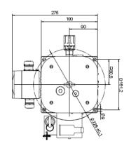
**Installation positions**BUEL® Model G thrusters have to be operated in vertical position (tank on top). A deviation of +/- 10° from the vertical axis is permitted.
