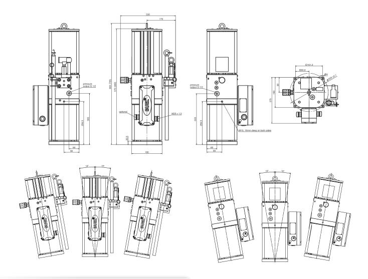
**Installation positions**BUEL® Model G thrusters have to be operated in vertical position (tank on top). A deviation of +/- 10° from the vertical axis is permitted.
