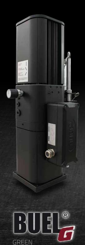
The BUEL® Model G is a new family member of the PINTSCH BUBENZER brand BUEL®. It is a compact thruster to feed active or passive hydraulic brakes and emergency brakes. It is also suitable for small capacity hydraulic cylinders. Operational pressure can be up to 250 bar.
