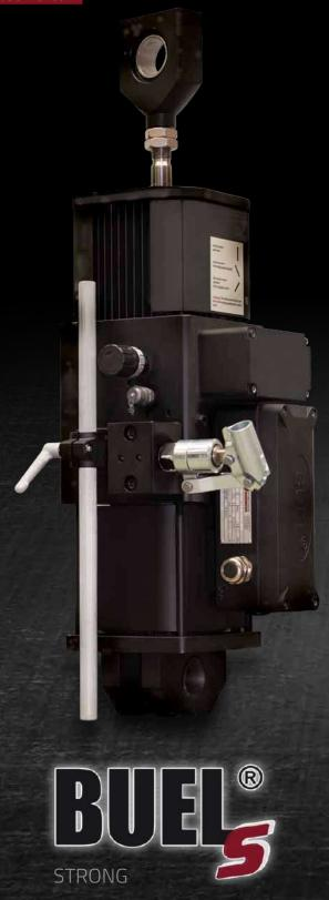
The BUEL® Model S is a brand new family member of the PINTSCH BUBENZER brand BUEL®. It is designed for wheel brakes on rail mounted cranes, where high pulling forces for mechanical wheel brakes are required. The patented cylinder system generates pulling forces up to 40.000 N. It has a robust, but also compact design for rough environmental conditions.
